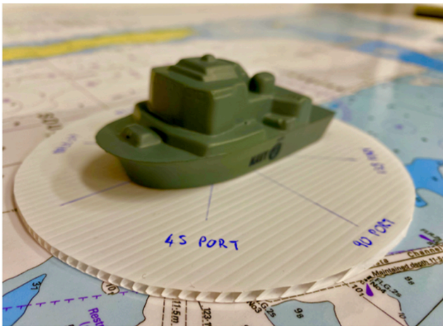
Fig. 4. The manual ATB tool used by OPTIX operators. Operators rotated the tool to match the orientation of a contact and used the bearing lines to inform estimates of ATB.
