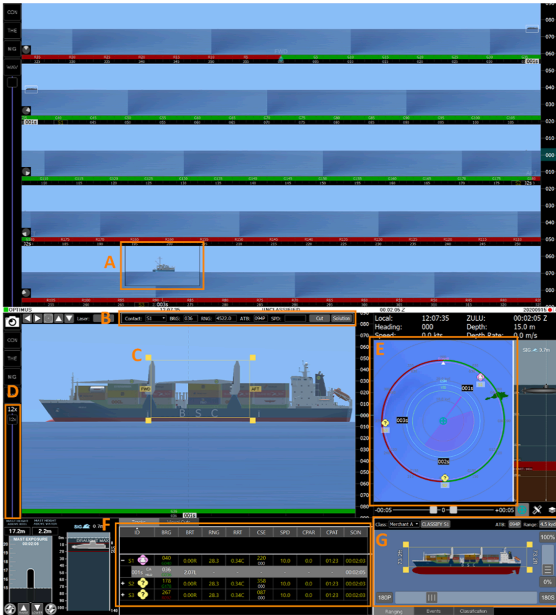
Fig. 3. The OPTIMUS HMI as presented on two vertically aligned screens, with key features marked. A: Magnified window, which could be controlled by mouse to inspect sections of the panorama. B: Visual cut window. The range and ATB (course) information in this window automatically updated as operators manipulated the yellow ranging box (C) and range/ATB tool (G). C: Ranging box in the analysis pane. Operators adjusted the position of the top and bottom lines to self-selected positions on the contact, and then matched these positions by manipulating the ranging box in the range/ATB tool (G) to generate a range estimate. D: Magnification slider for controlling magnification in the analysis pane. E: Geoplot showing a top-down view of the location and direction of travel of the submarine, and surrounding contact solutions. F: Contact tote listing the currently tracked contacts. G: Range/ATB tool showing a 3D model of the currently selected contact’s classification type. In addition to the ranging box described above, the slider at the bottom of this tool could be dragged to rotate the 3D model to match the visible contact. This generated an ATB estimate which automatically populated the visual cut window. The range/ATB tool could be toggled to the classification database in order to classify contacts. (For interpretation of the references to colour in this figure legend, the reader is referred to the web version of this article.)
